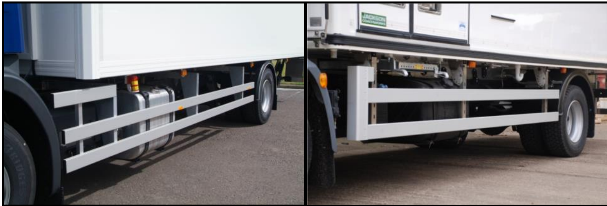
Figure 8. Left: Frame-mounted installation of a side guard. Right: Body-mounted side guard.
