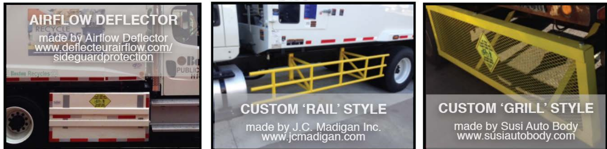
Figure 7. Boston’s side guard installation have been a mix of off-the-shelf (left) as well as custom fabricated models (center and right).
