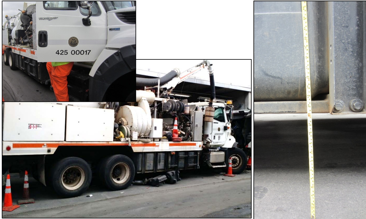
Figure 28. Examples of underbody equipment that already meets the recommended side guard dimensions.
