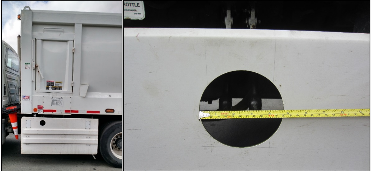
Figure 26. Access hole on this DPW side guard installation is well executed: small, smooth-edged, and away from the structural ribs of the fiberglass panel.
