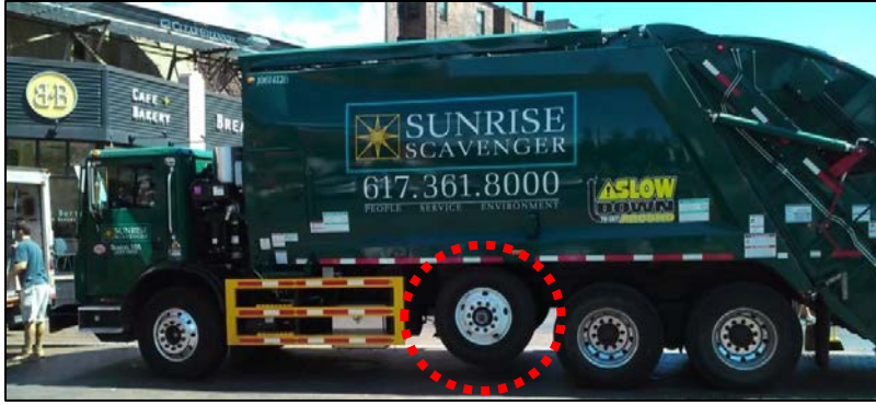
Figure 16. A Boston-based example of a tag axle that reduces the required length of the side guard.
