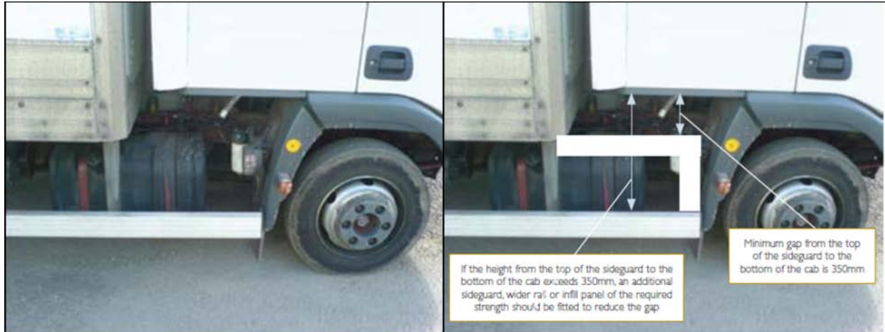
Figure 11. When the forward edge of the side guard falls under the cab, any gap between the cab and the top of the side guard exceeding 350 mm (13.5 in.) should be filled with an additional rail or panel of equal strength. 30
