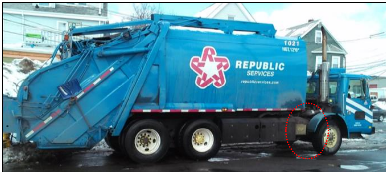
Figure 17. Example of installed underbody equipment on a DPW vacuum truck that achieves a flush, continuous surface and therefore the function of a side guard. No additional side guard is needed on this vehicle.
