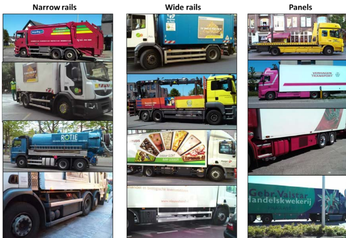
Figure 13. Either wide-rail or panel style side guards are recommended for maximum coverage and longitudinal
