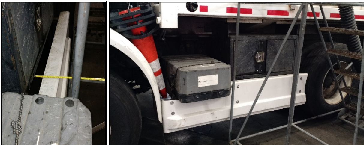
Figure 25. The recessed and protruding boxes do not provide a longitudinally smooth side guard surface. If possible, these should be realigned to be flush with the side guard. Additionally, the vertical gap over the forward box is excessive and should be covered (compare to example in Figure 11).
