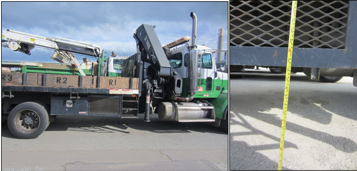
Figure 27. Expanded mesh panel side guard is well incorporated among other components but exceeds the recommended ground clearance.
