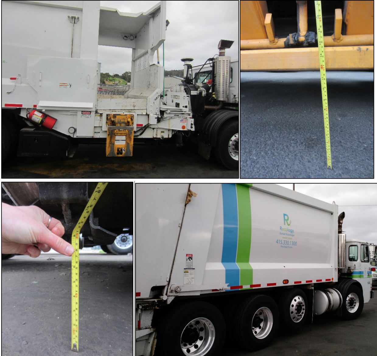
Figure 22. Wheelbase and ground clearance measurements on two Recology trucks. Top: 15 feet and 12 inches; Bottom: 13 feet and 7 inches.
