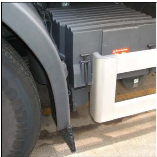
Figure 12. The forward edge of the side guard should have a continuous surface that turns inwards. This surface and turn-in is optional when the front edge of the side guard is within 100 mm (3.5 in.) of a permanent structure of the vehicle, e.g., cab or wheel arch. 31
