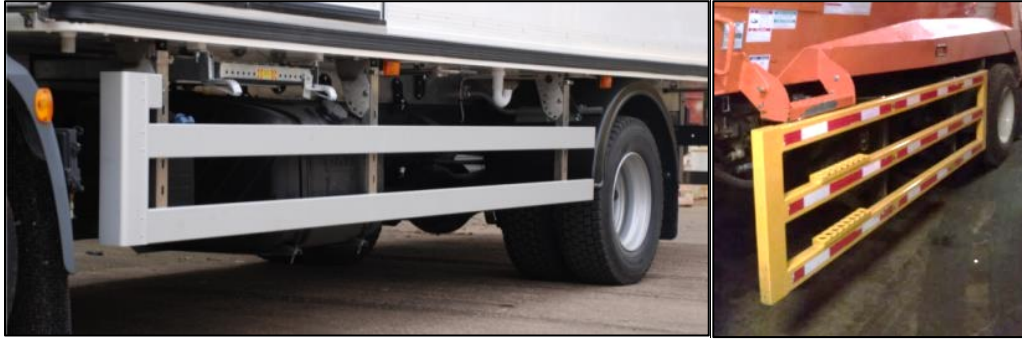
Figure 14. Wide, closely spaced rails on rail-style side guards (Left: UK example; right: Cambridge, MA example) are preferred over narrow rails.
