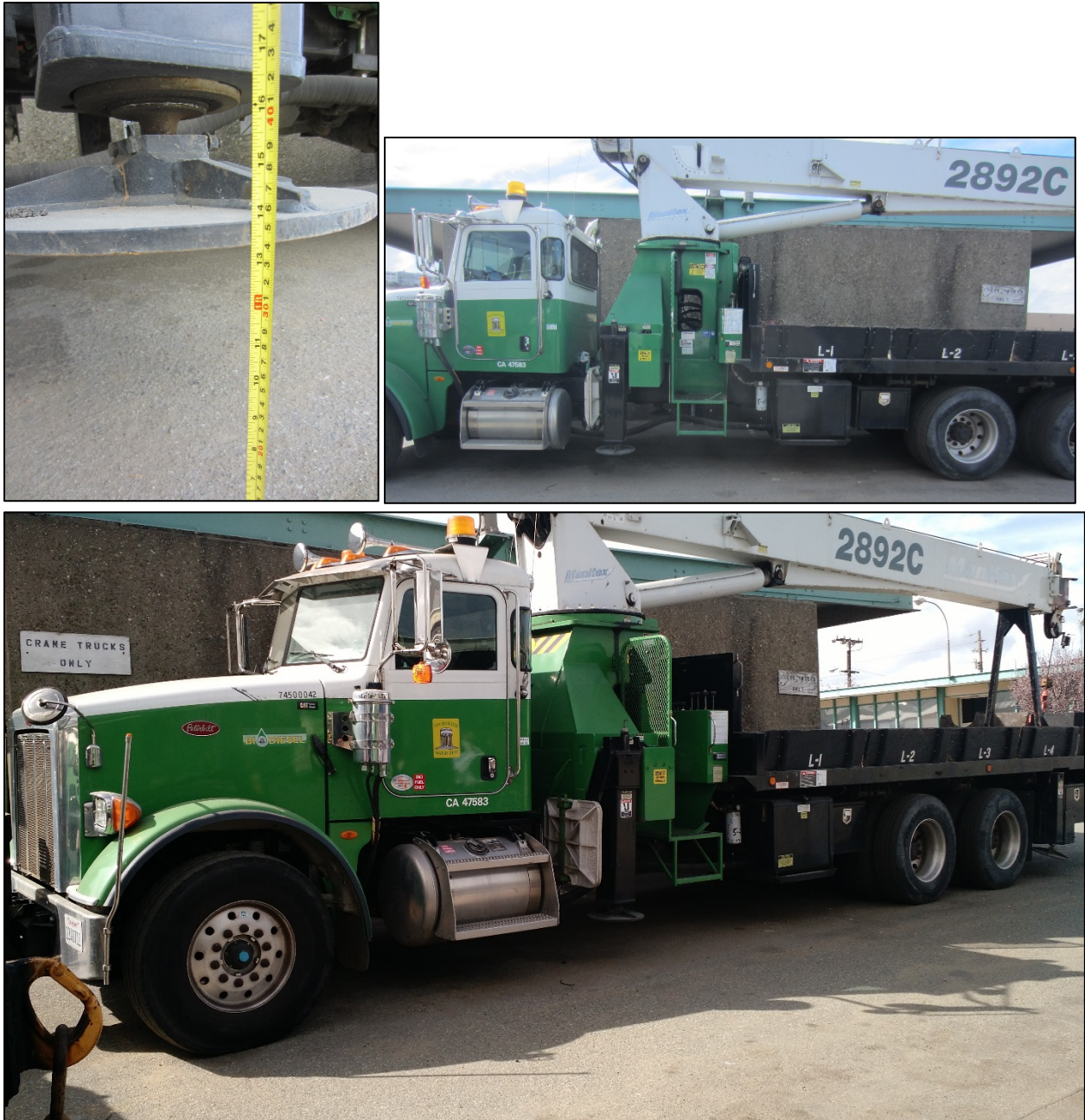
Figure 23. PUC Water wheelbase and ground clearance measurement: 21 feet and 13 inches.
