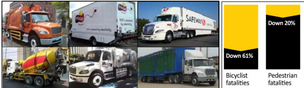
Figure 6. Diverse side guard designs are found globally, including a subset of aerodynamic side skirt models that also function as side guards. Right: Changes in the fatality rates of relevant side-impact crashes between VRUs and large trucks following the United Kingdom's passage of a national side guard law in 1986.
