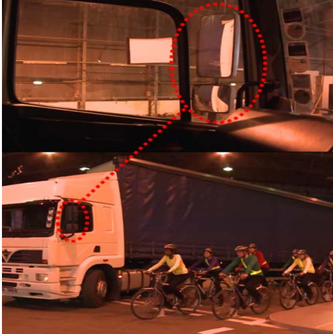
Figure 2. The blind spots of typical large truck mirrors, both planar and convex, can cover ten or more bicyclists or pedestrians. The operator can therefore be unaware of these road users when starting a turn. 7
